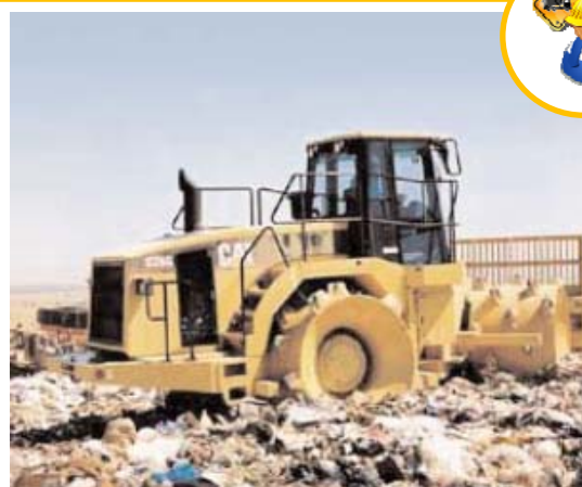
Steel wheeled compactors are used to move and compact waste at the working face (Photo courtesy of NSWMA)
