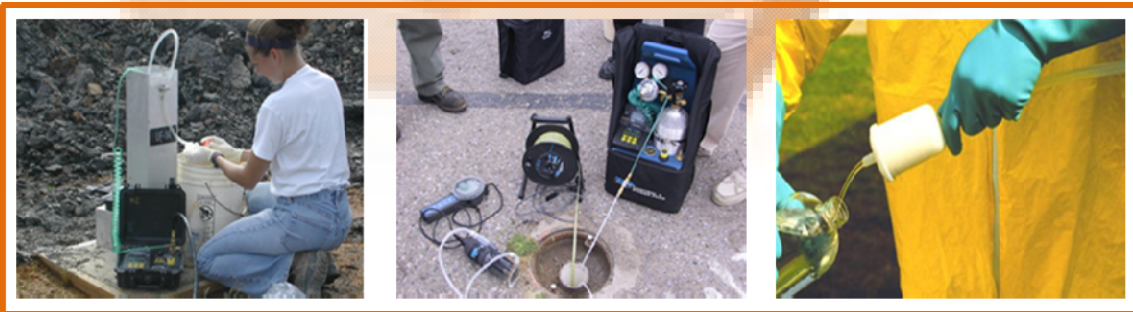
Testing of water samples in groundwater monitoring wells is used to demonstrate that the liner and leachate collection systems are working correctly to protect groundwater.
